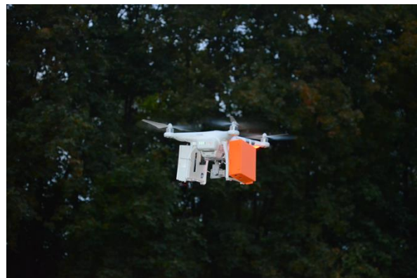
Figure 7. Lightweight aerometric platform mounted on a DJI Phantom 3 Advanced UAV during device testing on October 9, 2025, location - city park
