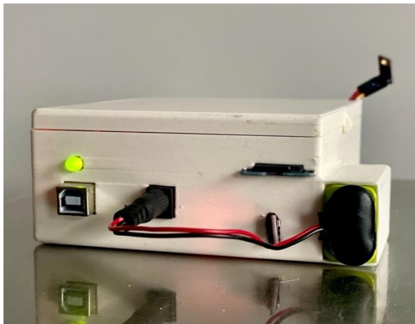
Figure 2. Lightweight measuring platform after printing and implementing the electronic circuit – final version, using Bambu Lab PLA Aero filament and a Bambu Lab A1 3D printer.
